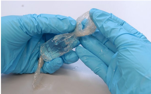
Figure 1. Tying a knot at the bottom and top of a dialysis membrane
