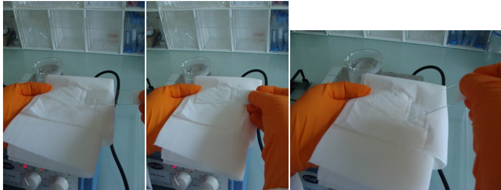
Figure 2. Slides coating with agarose. Removing of the agarose on the back of the slides.
