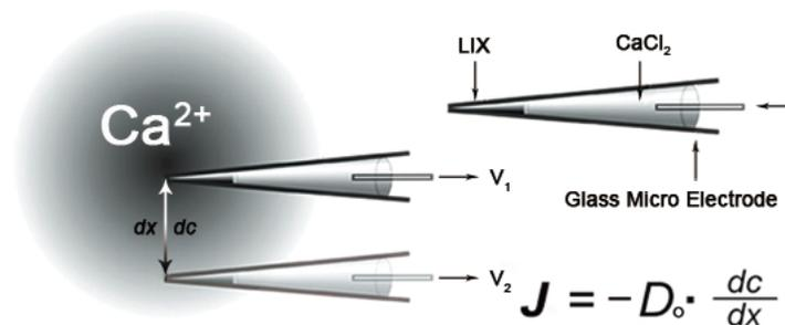
**Figure 1. Schematic diagram of ion flux detection ([www.xuyue.net](http://www.xuyue.net)). The microelectrode tip is filled with liquid ion exchanger (LIX). A voltage gradient ( $dV$ ) is measured by the electrometer between two positions over the travel range  $dx$ . A concentration gradient ( $dc$ ) is calculated based on  $dV$ .  $D_o$ , ion diffusion constant;  $J$ , net ion flux.**
