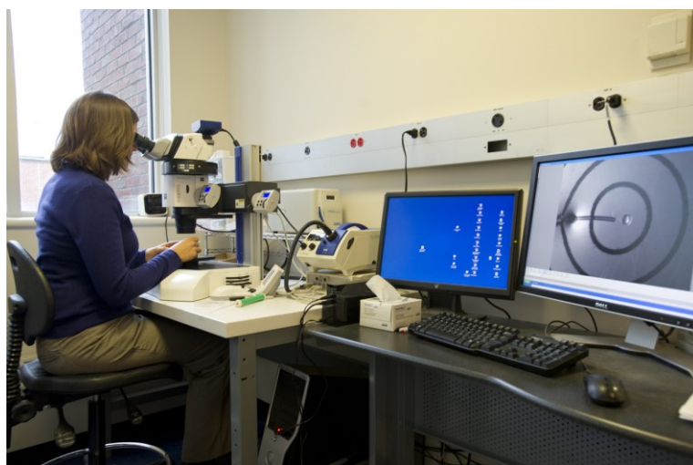
Figure 3. Microscope set up. A 60 mm Petri dish containing embryo media is placed on top of the motility wheel on top of the microscope stage. An embryo poker tool is used to position a zebrafish embryo in the middle of the motility wheel. Photo credit: University of Maine, Mike Mardosa.
