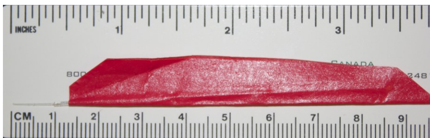
Figure 1. Embryo poker tool. This is a useful tool for the positioning and touch stimulus of zebrafish embryos. Fishing line (10 lb, 0.012 inch diameter) is super glued into the end of a glass capillary tube (Sutter Instruments, catalog number: BF100-50-10) with approximately 1 cm of overhang. The glass capillary tube is then wrapped in lab tape.
