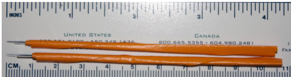
Figure 1. Deyolking tools. Deyolking tools can be used to surgically remove the yolk sac from fixed zebrafish embryos. Deyolking tools consist of insect pins (fine Science Tools, catalog number: 26002-20) super glued into the ends of glass capillary tubes (sutter Instruments, catalog number: BF100-50-10). The glass capillary tubes are then wrapped in lab tape.
