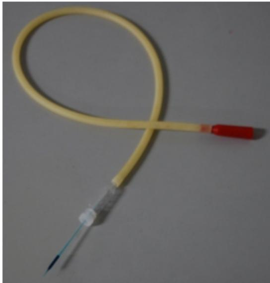
**Figure 1. An aspirator tube and a glass capillary**
