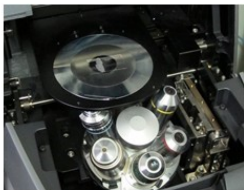
Figure 7. A cover glass placed on the microscope stage. In this case, imprint is placed on the upper surface of the cover glass for imaging on inverted microscope.
