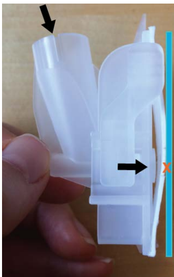
Figure 1. Image showing the cytofunnel. Top arrow indicates the site of loading into the funnel. Bottom arrow indicates the flow direction of the cell suspension toward the slide, which
