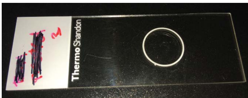
Figure 2. Image of the cytospin slide. The sample is within the white circle. A round coverslip covers the area within the circle and nail polish is used to seal the coverslip along the edges/the white circle.
