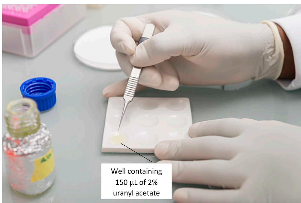
Figure 2. Photo on how to float the carbon film into a well containing the negative stain solution
