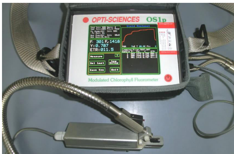
Figure 5. OS1p-Chlorophyll fluorometer. The display shows three exemplary measurements down right and general settings top left. Besides this, the leaf clip for measurement is shown consisting out of the clip with the trigger button and the sensor for detecting the photosynthetic active radiation (PAR).
