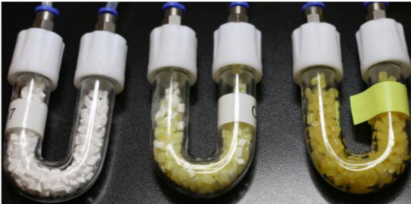
Figure 1. A photo of the U-shaped Pyrex tube filled with microporous granules showing different levels of saturation with Carvon odor solution. From left to right: pure granules without any added odor solution; partly saturated granules; fully saturated granules as used for the experiments.
