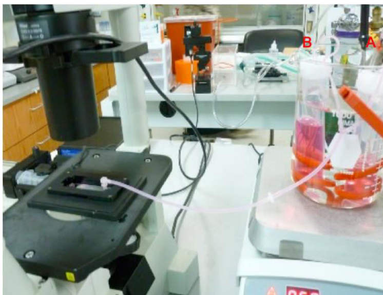
Figure 9. The process of line washing with culture medium via line connected to Reservoir B
