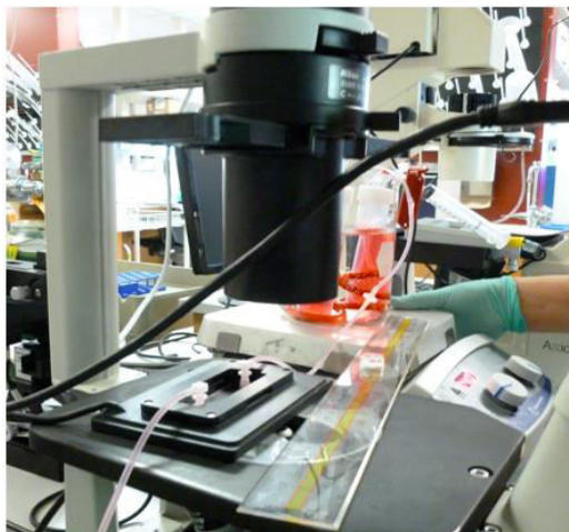
Figure 11. Leveling the heights of chamber and reservoir
