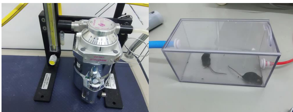
Figure 1. Anesthesia of animals. Mice are placed in an anesthesia chamber (ideally red transparent) and oxygen/inhalation anesthetic flow is controlled.
