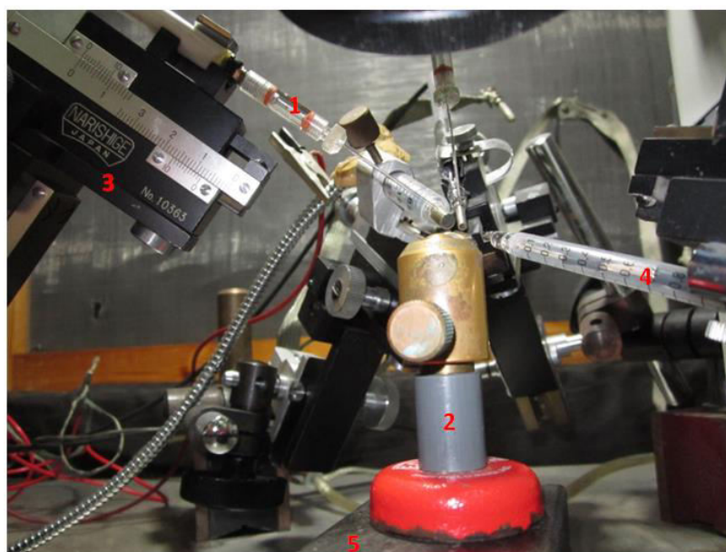
Figure 2. A magnified view of the ERG setup: #1-electrode holder, #2-fly stand, #3-micromanipulator, #4-light detector probe, #5-magnet block
