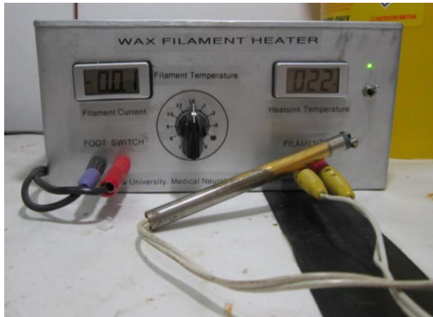
Figure 3. A homemade instrument for immobilizing the living fly: A platinum-iridium (0.25 mm diameter) filament is electrically connected to a power supply with a controlled current output. The filament is attached via insulating plastic to a copper rod holder (heater and soldering iron)
