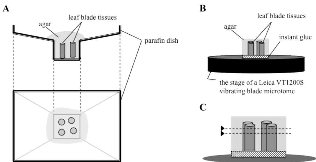
**Figure 2. Schematic drawing of section preparation.** Rice leaf blade tissues are embedded in agar (A), and the agar block is glued on the stage of a Leica VT1200S vibrating blade microtome (B). The agar-embedded tissue is cut parallel to the surface of the stage (shown as dotted lines in C).
