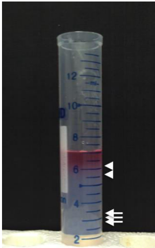
Figure 5. An example of Percoll gradient. Arrowhead; Schwann cell layer; Arrow; DRGs layer.
