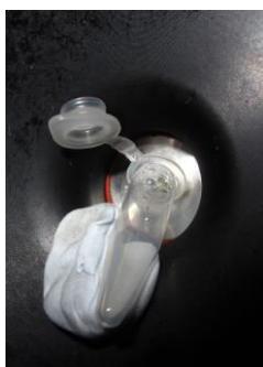
Figure 2. An example of xylem sap being collected from a sample enclosed in a Scholander pressure chamber. The collection tube can be held in place with Blu-Tack or modeller's clay.
