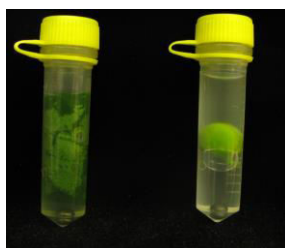
Figure 4. Leaflet tissue of the angiosperm Pisum sativum (left) (taken from Figure 1) and a green seed of Pisum sativum (right) enclosed in 2 ml screw-top tubes and covered in cold 80% methanol with added BHT. Note the stainless steel bead that has already been added to the tube at the bottom, and the correct tethering of the tube (a step critical for successful long-distance freight).
