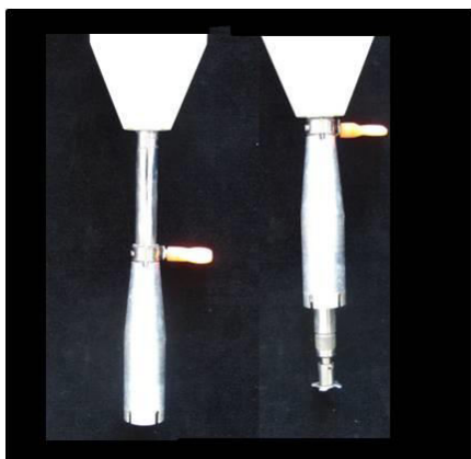
Figure 5. Modified Ba-Mix ® for homogenizing plant tissues in a 50 ml centrifuge tube. Note the movable aluminium sleeve, the right-hand image shows the sleeve fully raised exposing the modified blade. The blade of this Ba-Mix ® spins at high speed and, if the sleeve is moved up and down while homogenizing, the sample is forced through the spinning blade and is macerated. It is important that the tissue is forced passed the blade by adjusting the height of the sleeve relative to the blade.
