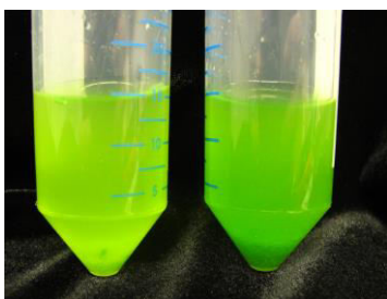
Figure 6. An example of the degree of homogenization after the use of a Physcotron on the samples of the conifer Callitris rhomboidea (left) and angiosperm Olea europaea (right) shown in Figure 4. Note the increase in liquid from rinsing the homogenizer in 80% methanol in water after use.
