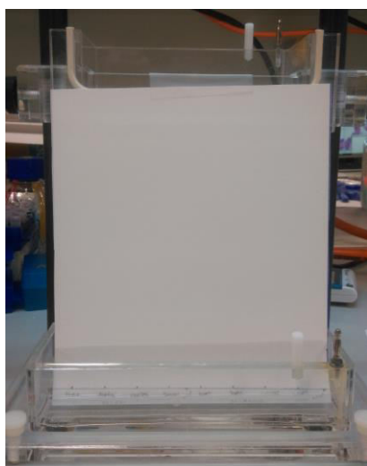
Figure 3. Setup the TLC chamber with the PEI-cellulose TLC plate containing the migration buffer (composition in step 7)
