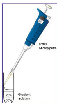
Figure 1. Illustration showing the way to layer the gradient solution using P200 micropipette. Pour 360 \mu l of each gradient solution carefully into a centrifuge tube using P200 micropipette (180 \mu l x 2 times), not to make bubbles nor disturb the other layers. Layer in a centrifuge tube from the heaviest (30%) to lightest (5%) solution.
