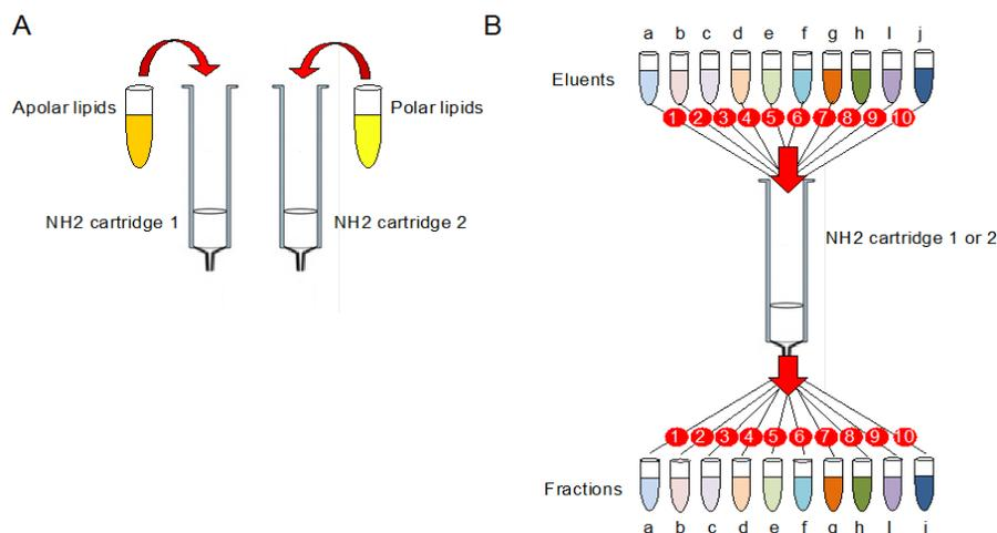
**Figure 1. Scheme illustrating the lipid fractionation procedure.** A. Loading of apolar and polar extracted lipids on two separate amino (NH<sub>2</sub>) cartridges. B. Sequential elution of lipid fractions from the amino cartridges. Letters indicate eluents and corresponding fractions. Numbers indicate the temporal order of elution and fraction collection.
