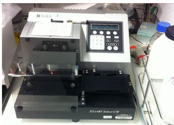
**Figure 1. Picture of plate washer**
