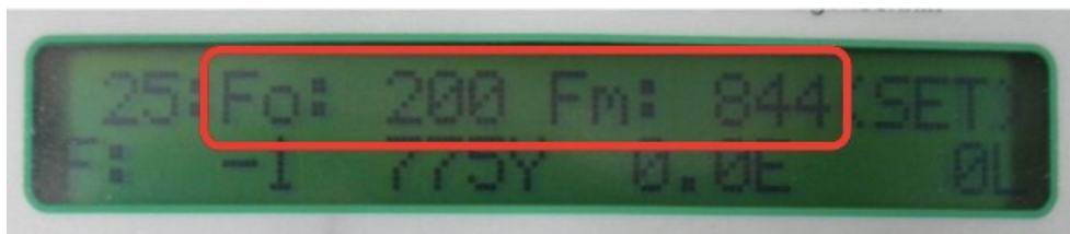
Figure 5. A photo of the display when setting Fo and Fm ("Mode" menu 25)
