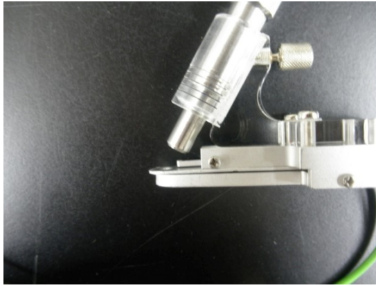
Figure 3. A photo of the leaf clip holder and fiberoptics
