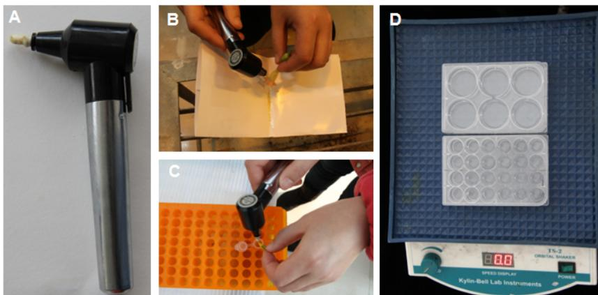
**Figure 1. Pollen collection and liquid germination assay.** A. An image of a biovortexer. B-C. Mature pollen of tobacco (B) or tomato (C) was collected by vibrating using a biovortexer. D. Pollen in germination medium was transferred to a 6 well culture plate (~2 ml/well) or a 24 well culture plate (0.5 ml/well) and germinated on an orbital shaker under fixed room temperature.
