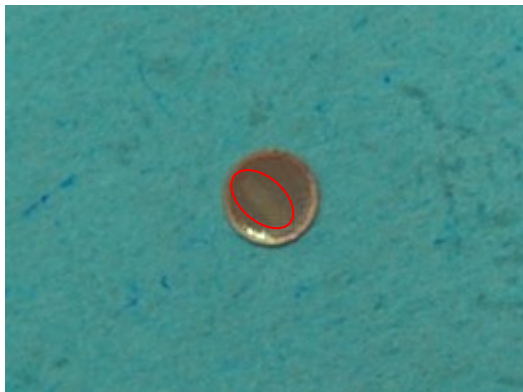
Figure 1. A picture of copper grid with sample sections. The red circle indicated the sample sections.
