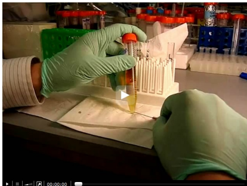
Video 1. Removal of lipid phase from plastic tube. The video shows how to insert a needle into the polypropylene tube and drain the lipid phase from the tube.
