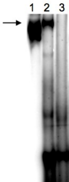
Figure 2. Scanned image of native PAGE gel after binding assay. This is an example of the separation of unbound, small tRNA* at the bottom of the gel and the tRNA* bound to the much bigger T-box RNA (arrow), which was transcribed in vitro in the presence of pre-formed, radiolabelled(*) tRNA. lane 1: control IVT reaction of T-box RNA* without tRNA; lane 2: T-box RNA IVT with tRNA*fMet; lane 3: T-box RNA IVT with tRNA*Cys (not binding to T-box RNA).
