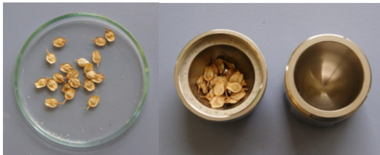
Figure 2. 20 ripe fruits of L. campestre (left) placed in a grinding jar of the mixer mill together with six 5-mm steel balls (right)
