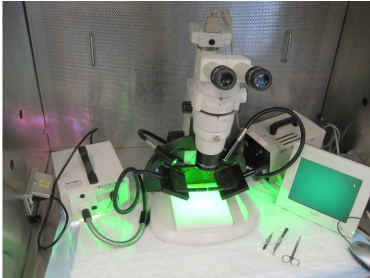
Figure 1. Equipment required to visualize and collect GFP-MSC aggregates/spheres from the mouse peritoneum. GFP-MSC aggregates/spheres can be visualized in the mouse peritoneum using a dissection microscope with an epi-fluorescence attachment and GFP filter set. High quality images can be acquired with an appropriate camera mounted to the dissection scope (A camera is not a requirement for collecting the aggregates.).
