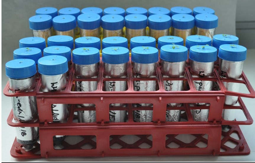
Figure 1. Falcon tubes with single seedling each – ready to determine Falcon weight at the beginning of experiment (W0)
