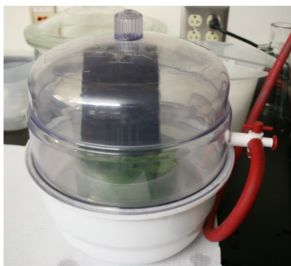
Figure 1. Vacuum Infiltration. The mAb vector is delivered via A. tumefaciens into N. benthamiana leaves using vacuum infiltration (see above, procedure step 7).
