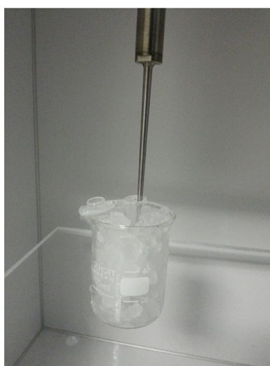
Figure 2. Cells sonication. Sonication was performed to dissolve cells aggregate. During sonication the tube is kept in ice to minimize protein denaturation.
