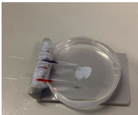
Figure 5. Electrodes stored in BSM solution
